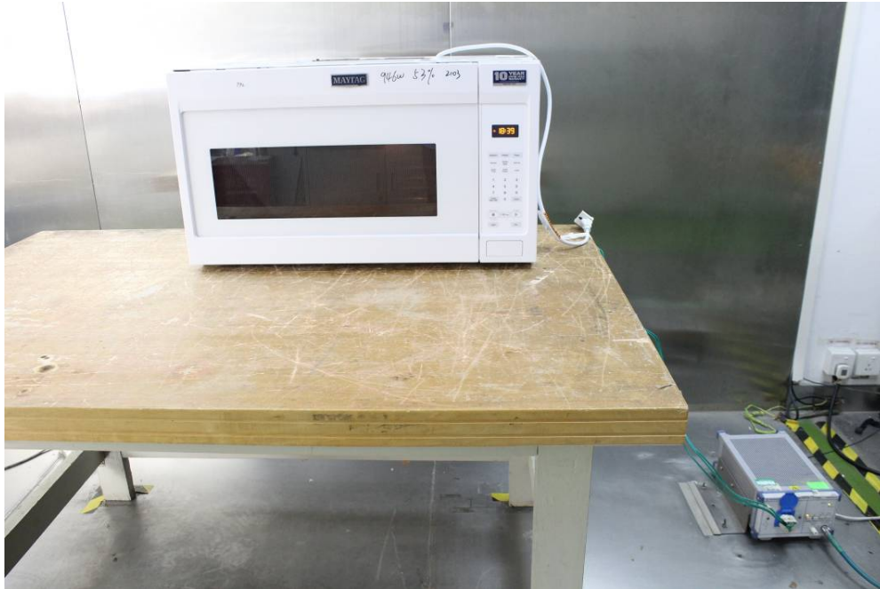
Conducted Emissions - Front View
