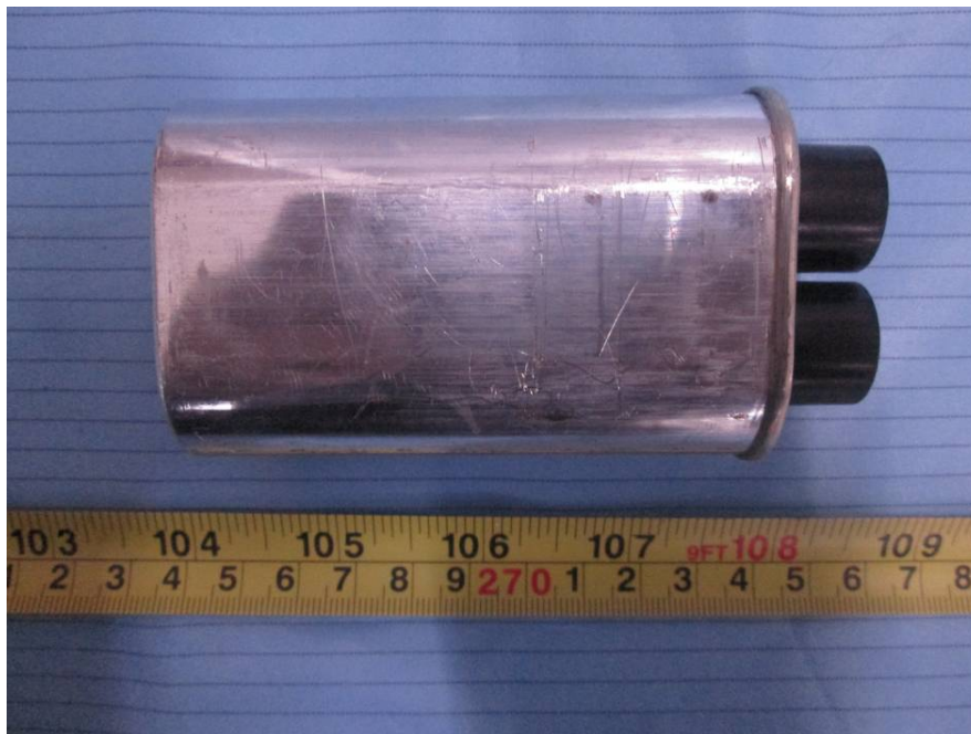
EUT – H.V. CAVAPTOR Bottom View
