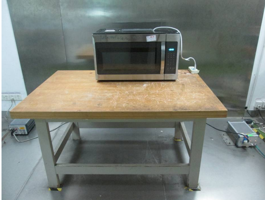
Conducted Emissions - Front View
