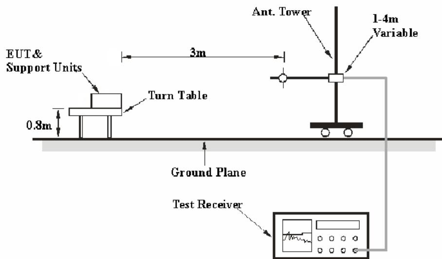
The radiated emission tests were performed in the 3 meters chamber A test site, using the setup accordance with the FCC MP - 5. The specification used was FCC part 18 limits.
