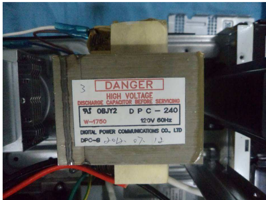
EUT – Transformer View (Option-2)
