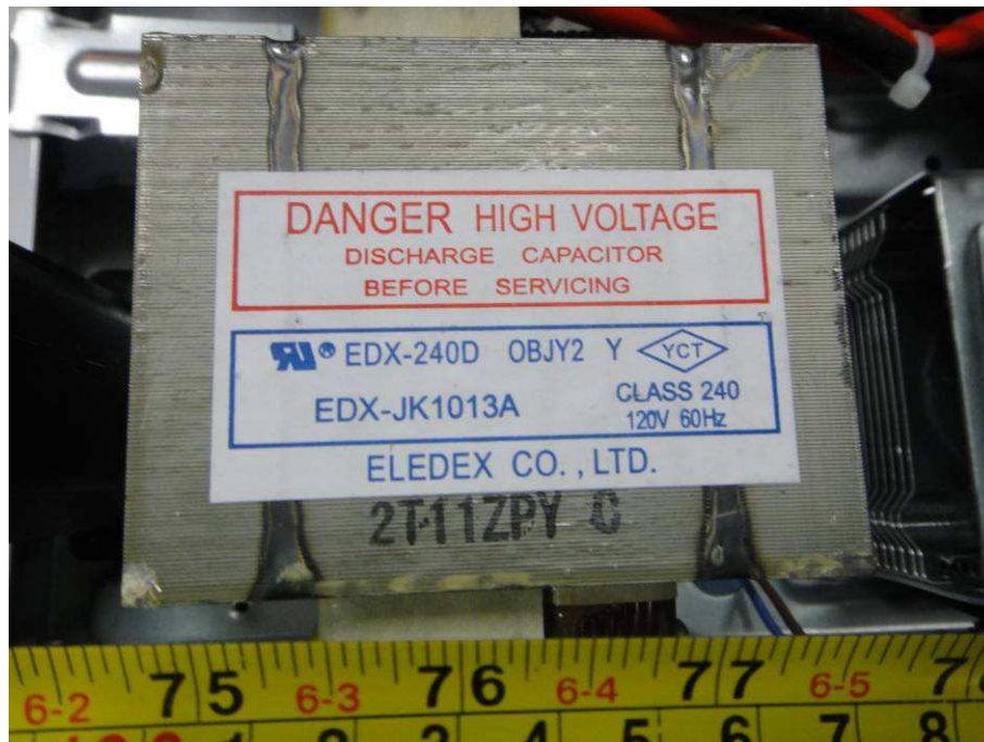
EUT – Transformer View (Option-1)
