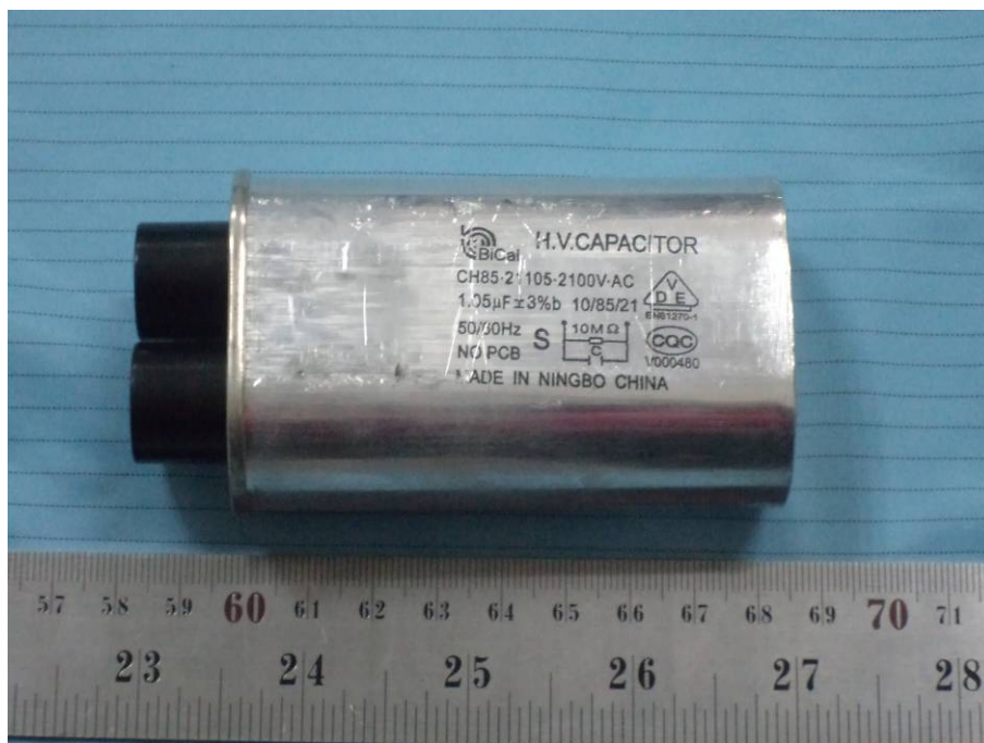
EUT – HV Capacitor View
