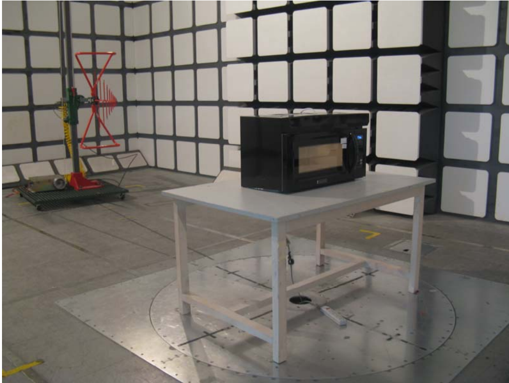
Radiated Emissions-Rear View (30 MHz-1000 MHz)
