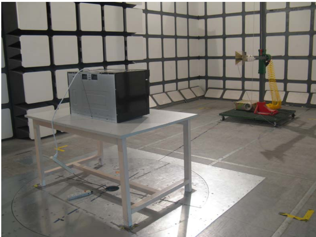
Radiated Emissions-Rear View (Above 1 GHz)
