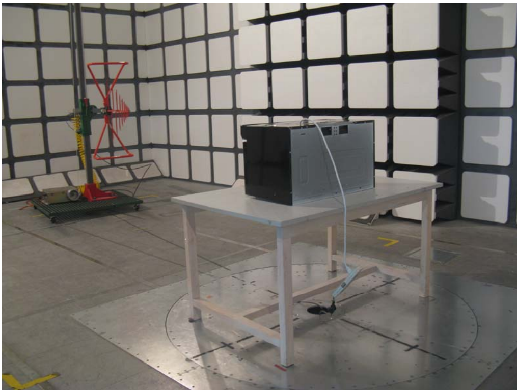
Radiated Emissions-Rear View (30 MHz-1000 MHz)
