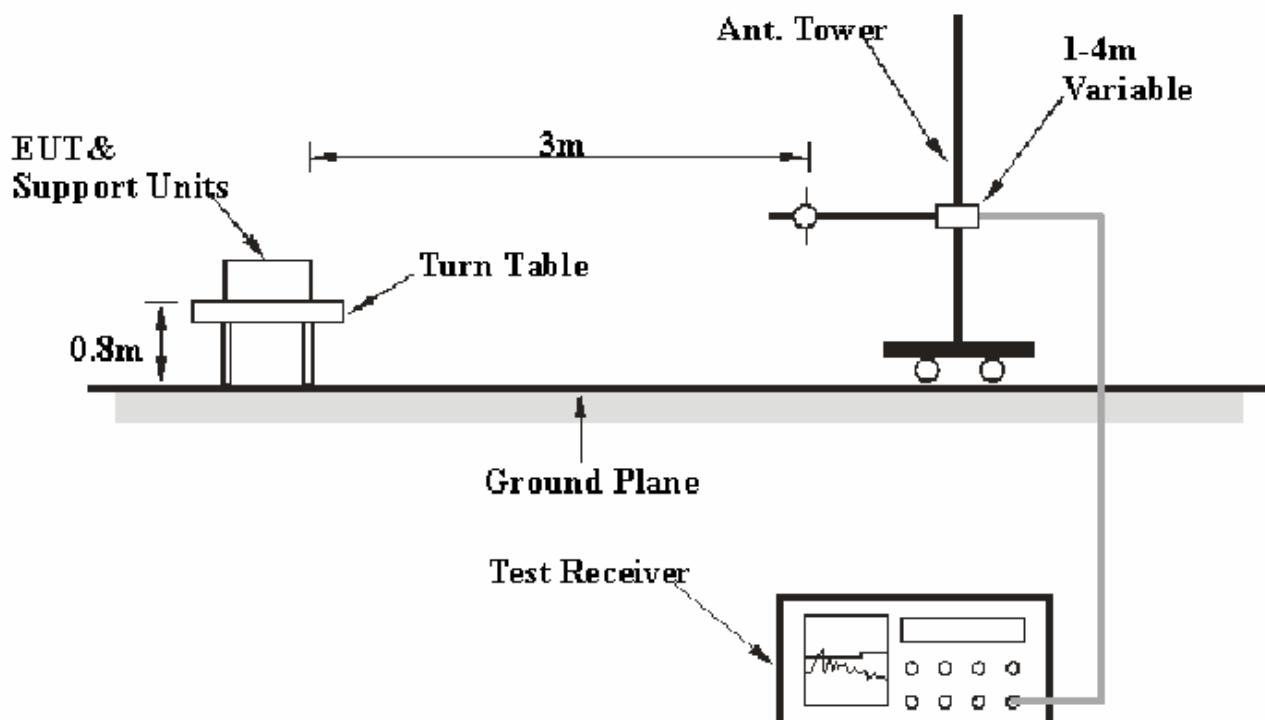
The radiated emission tests were performed in the 3 meters chamber B test site, using the setup accordance with the FCC MP - 5. The specification used was the FCC part 18 limits.
