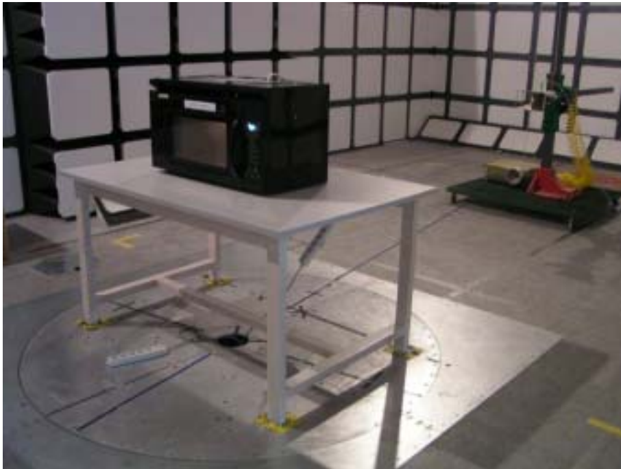
1000 MHz to 25GHz: Radiated Emissions-Front View
