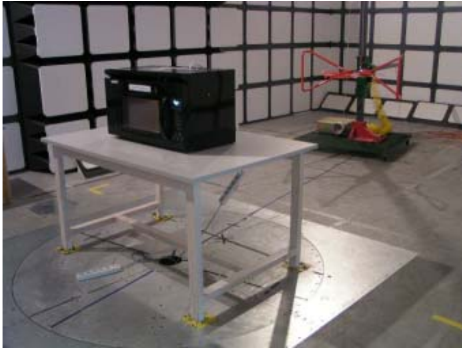
30 MHz to 1000MHz: Radiated Emissions-Front View
