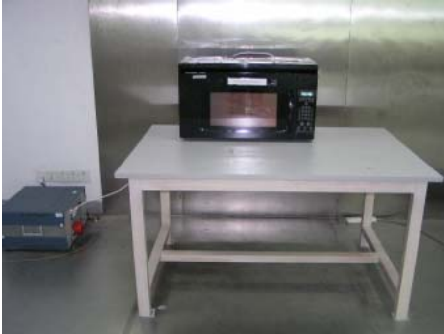
Conducted Emissions-Front View
