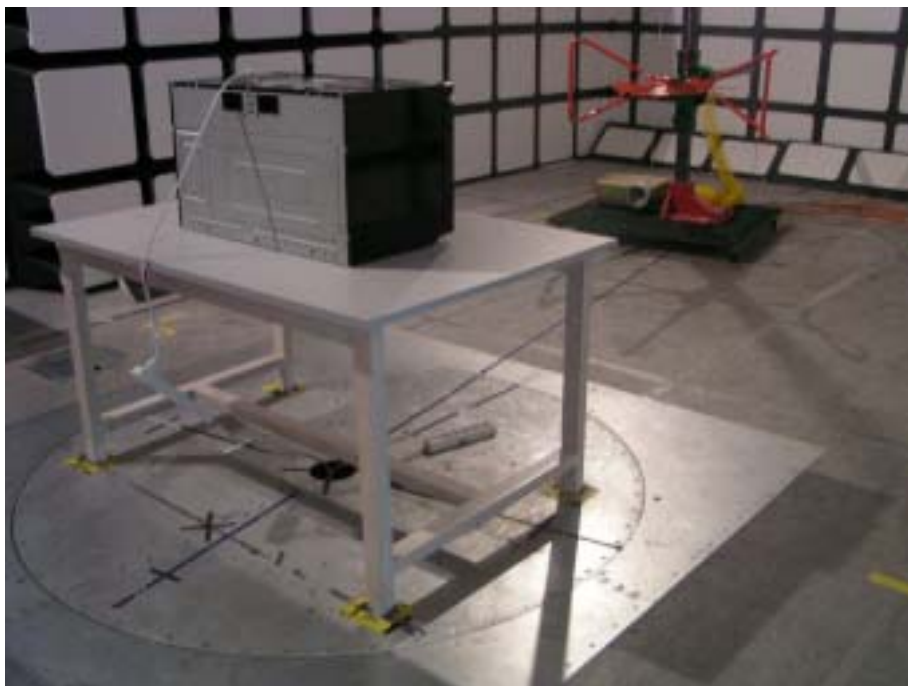
30 MHz to 1000MHz: Radiated Emissions-Rear View
