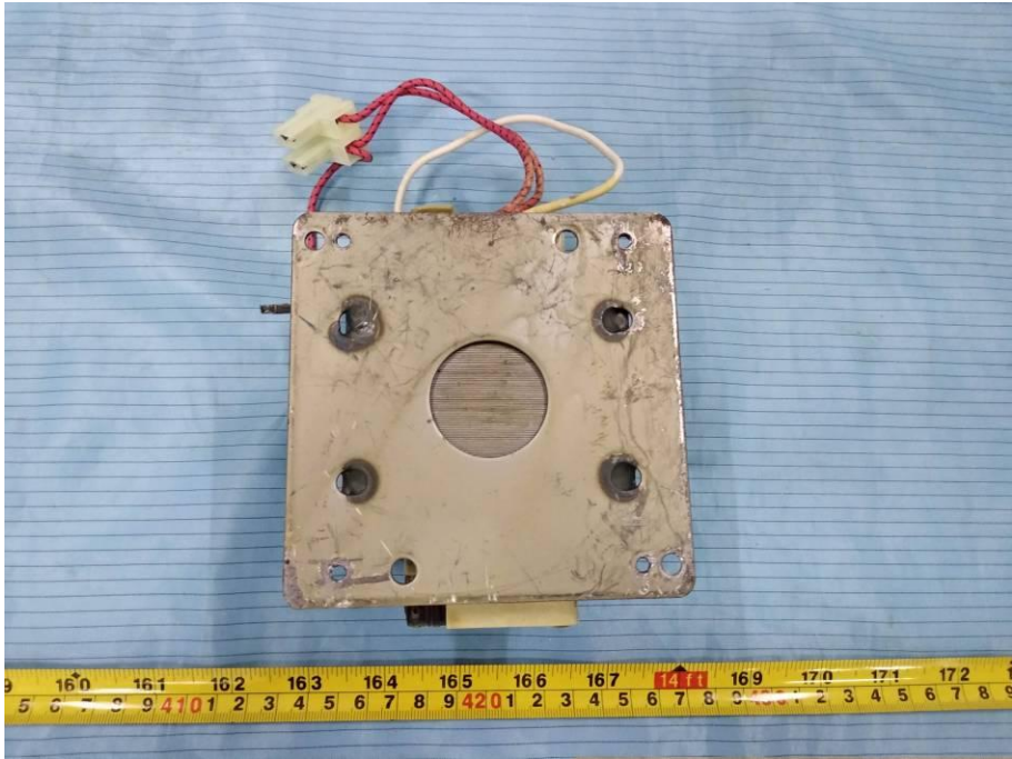
EUT – Transformer 1 Bottom View
