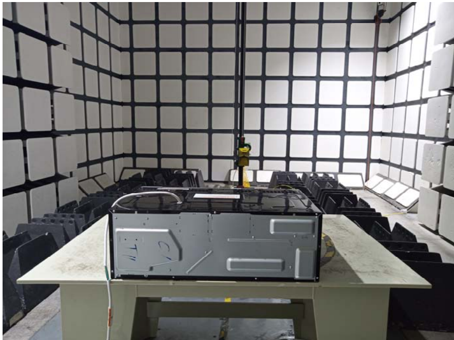
Radiated Emissions - Rear View (Above 1 GHz)
