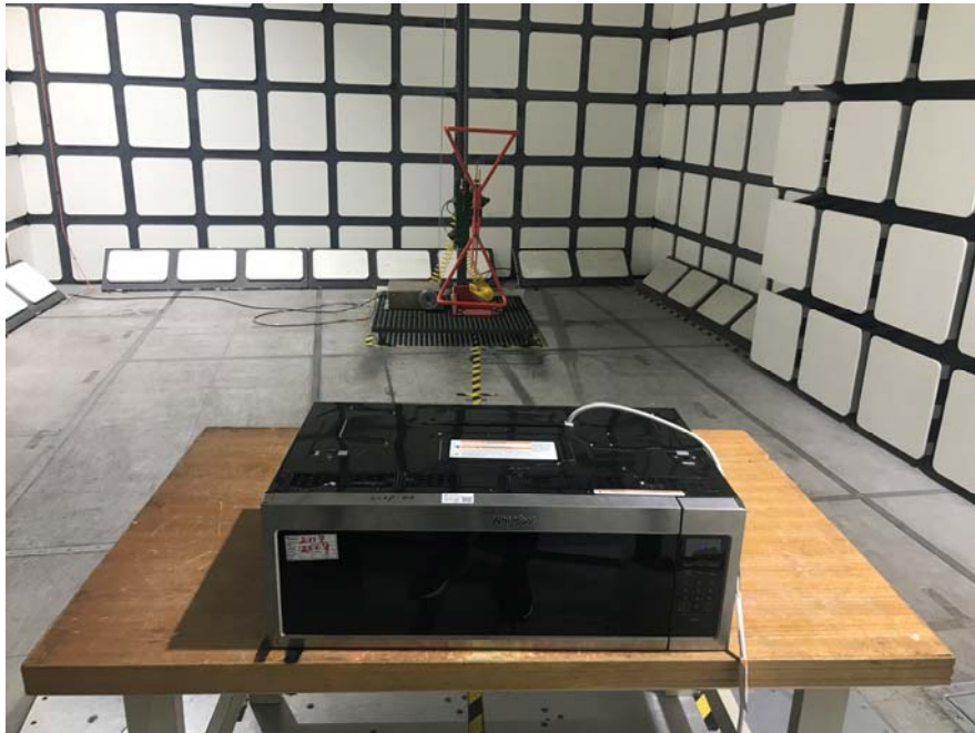
Radiated Emissions - Rear View (30 MHz – 1 GHz)
