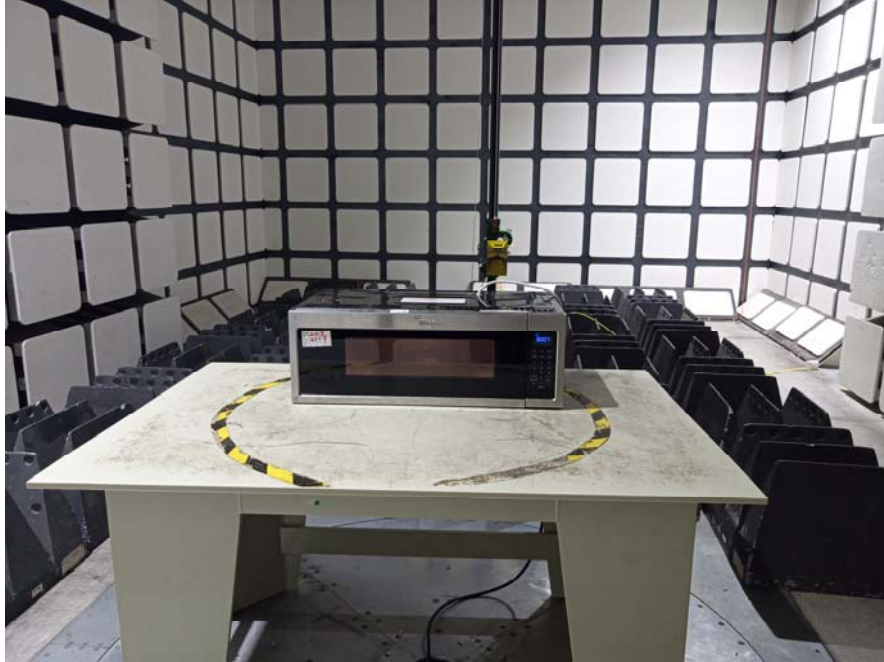
Radiated Emissions - Front View (Above 1 GHz)
