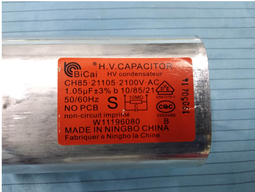
EUT – H.V. Capacitor Label View
