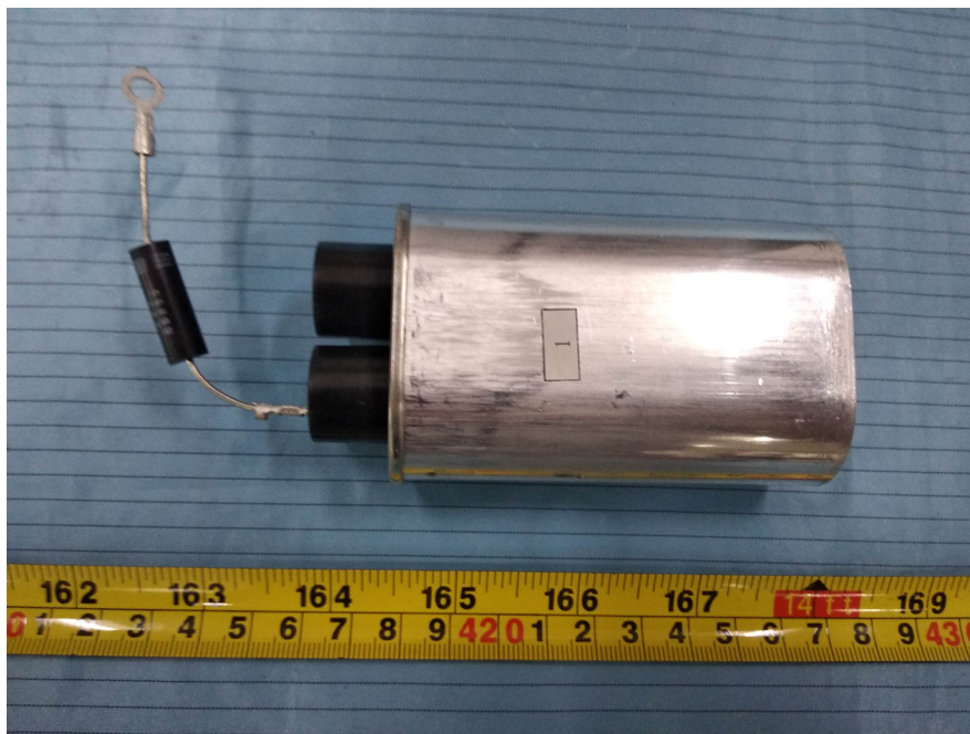
EUT – H.V. Capacitor Bottom View
