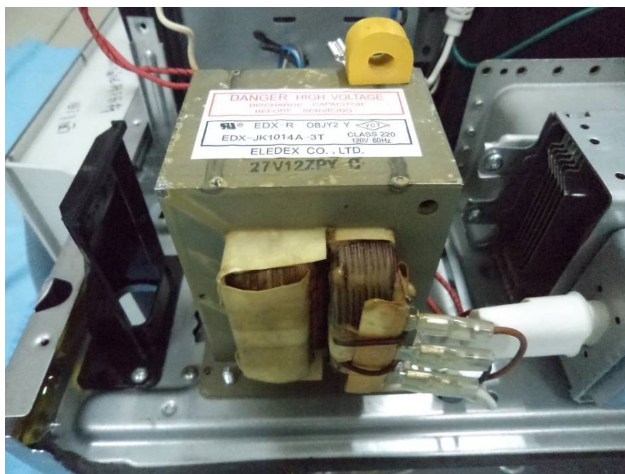
EUT – Power Transformer View
