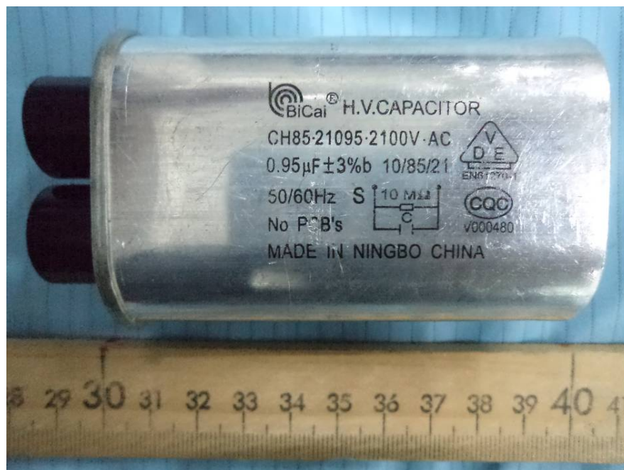
EUT – H.V. Capacitor View
