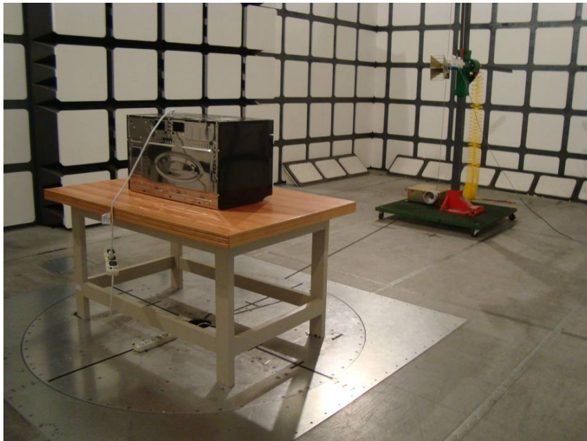
Radiated Emissions - Rear View (Above 1 GHz)
