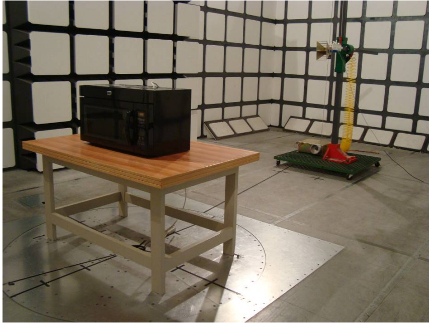
Radiated Emissions - Front View (Above 1 GHz)
