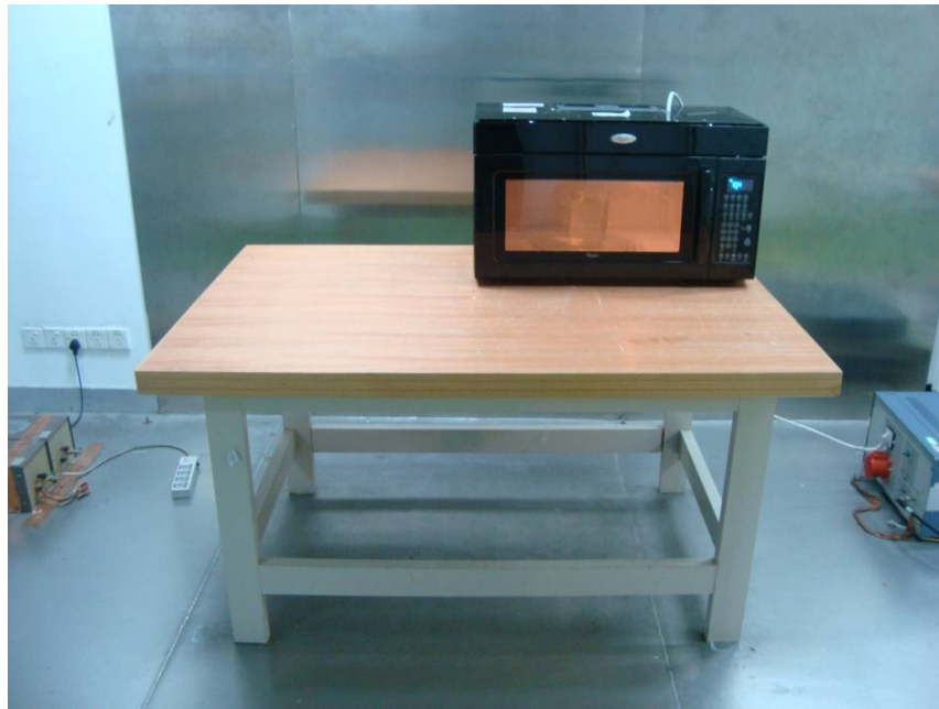
Conduction Emissions - Front View
