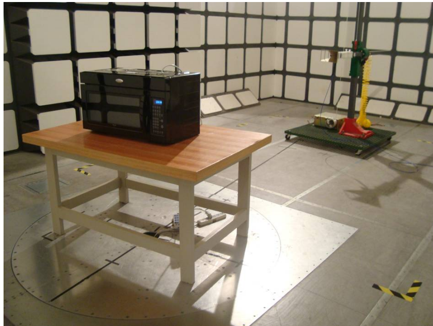
Radiated Emissions - Front View (Above 1 GHz)
