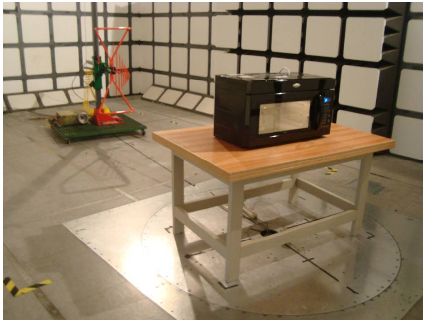
Radiated Emissions - Front View (Below 1 GHz)
