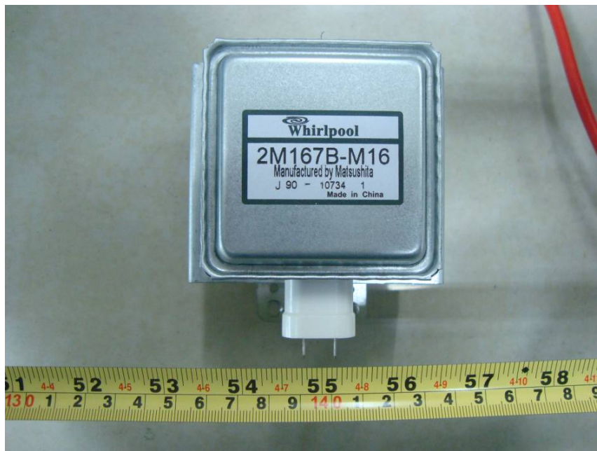
EUT – Magnetron View
