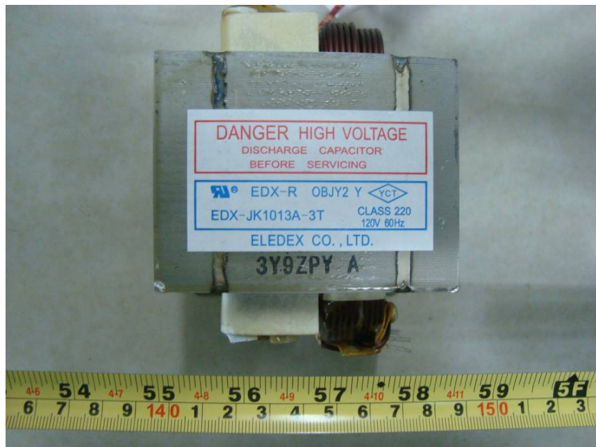
EUT – Transformer View
