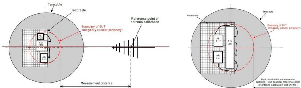
The radiated emission tests were performed in the 3 meters chamber test site, using the setup accordance with the FCC MP - 5. The specification used was the FCC part 18 limits.
