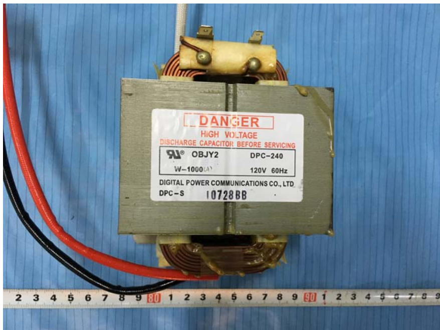
EUT – Transformer View
