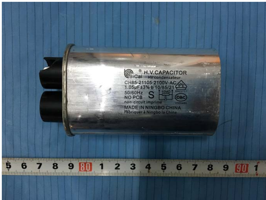
EUT – H.V. Capacitor View
