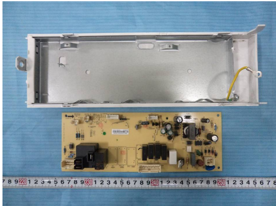
EUT –Control Panel Cover off View
