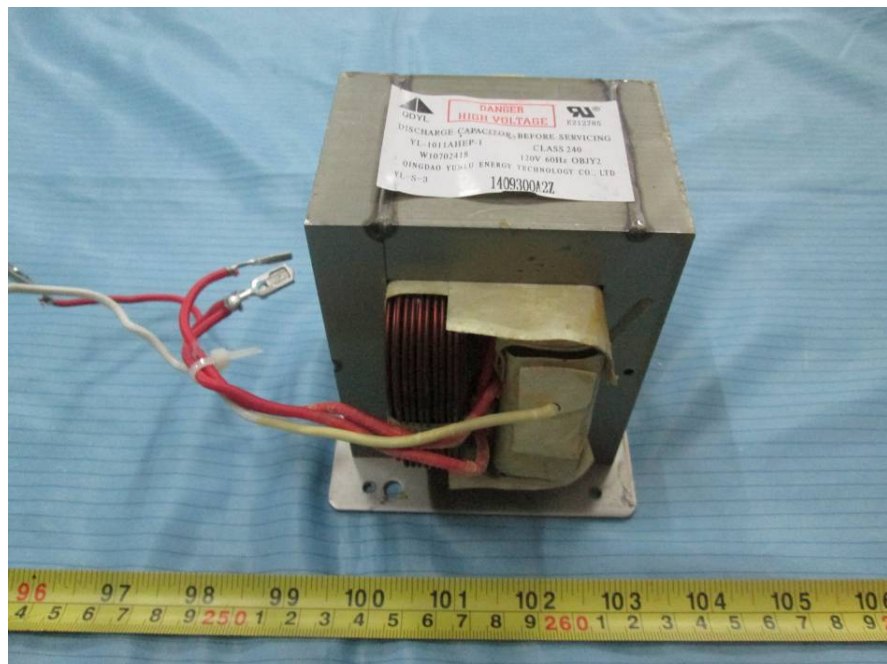
EUT – High Voltage Transformer View
