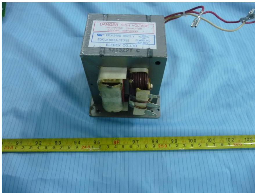
EUT – Power Transformer View
