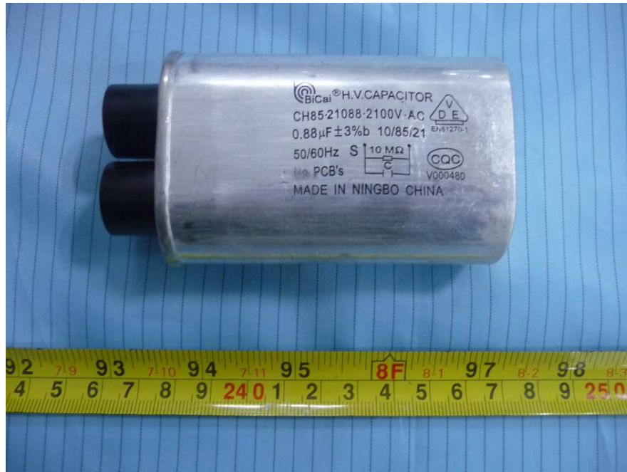
EUT – H.V. Capacitor View
