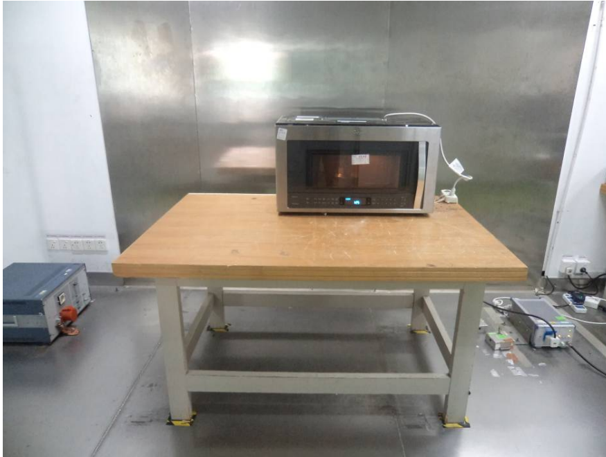
Conducted Emissions - Front View
