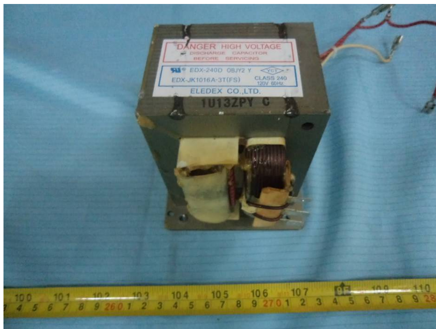
EUT – Power Transformer View
