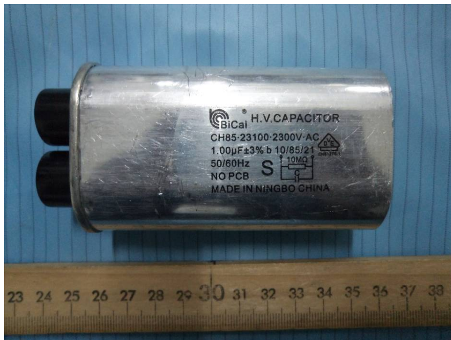
EUT – H.V. Capacitor View
