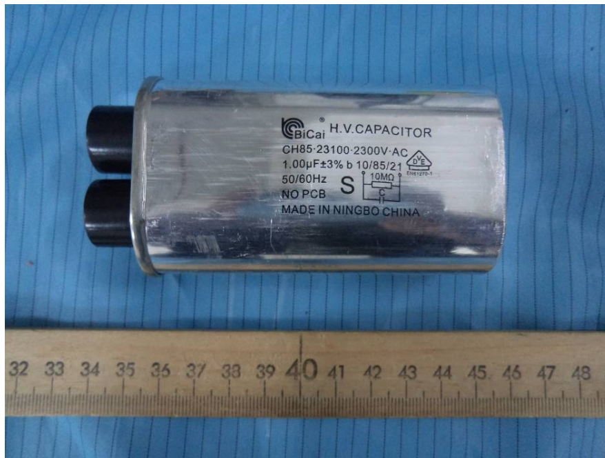
EUT – H.V. Capacitor View
