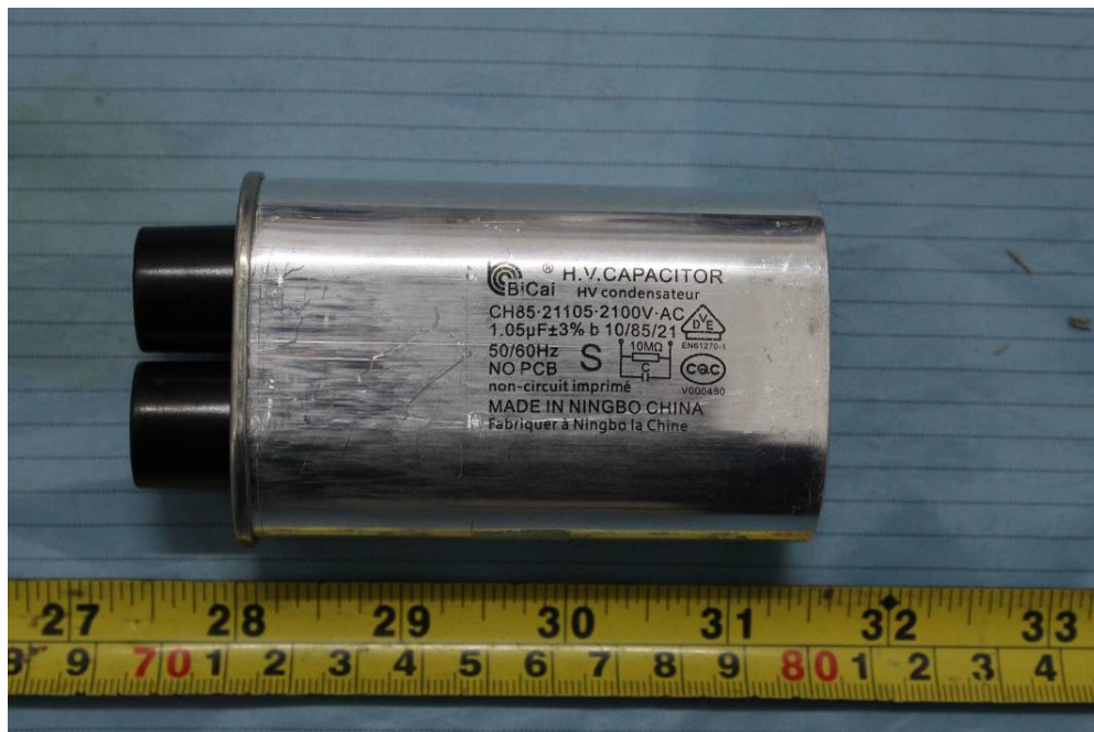
EUT – H.V. Capacitor View
