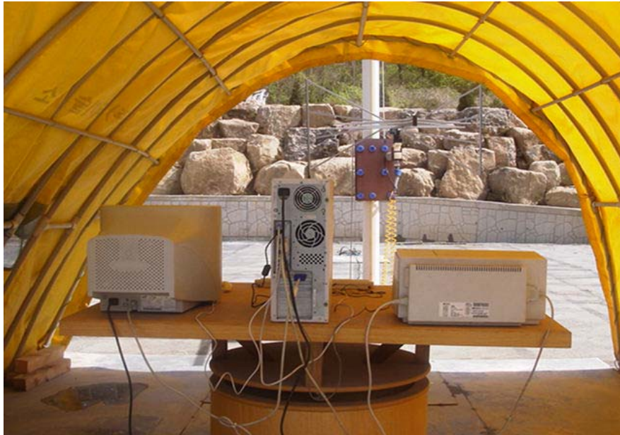
Photograph 1 : Setup for radiated Emissions
