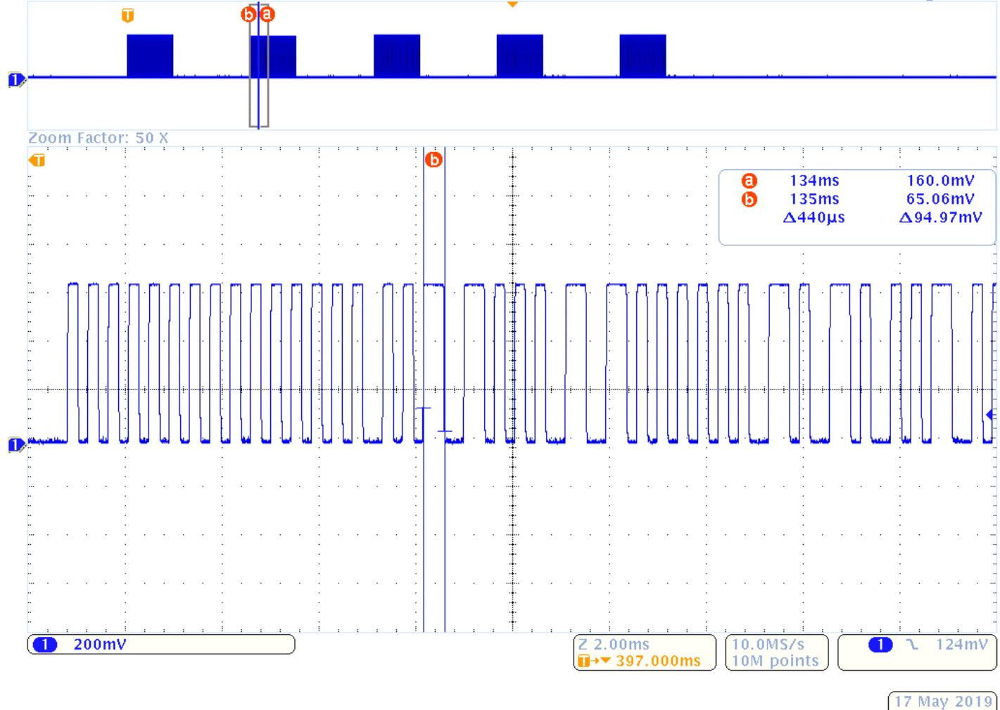
Test Method: FCC Part 15.231(b), Duty Cycle Determination
