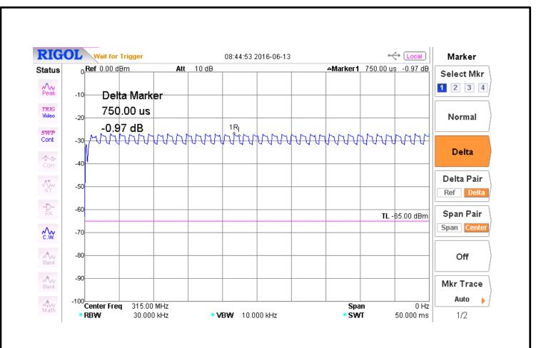
Test Method: FCC Part 15.231(b), Duty Cycle Determination IC RSS-210 A1.1.2(2) Pulsed Operation Notes: Narrow Pulse Width On Time = 750.0 uS
