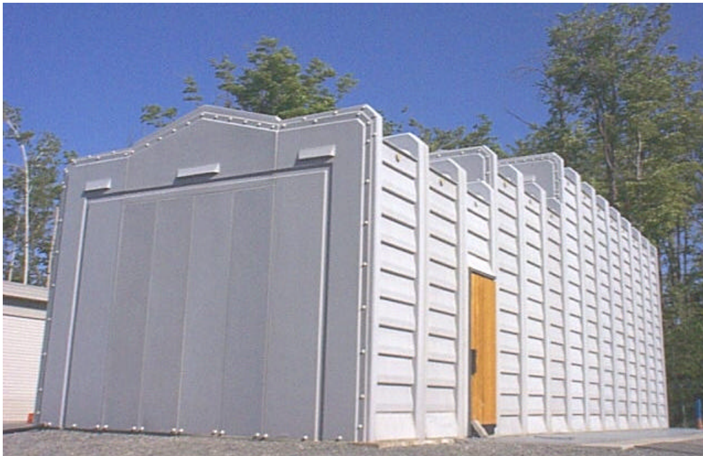
Fig. 1.b APREL's OATS (Open Area Test Site)
