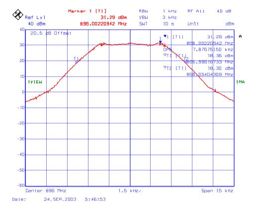
Plot # 3: 99% OBW, RF Output Frequency: 898.5 MHz, Modulation: 2-Level 8kbps GMSK
