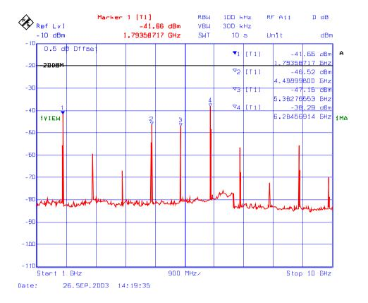
Plot # 21 : Spurious Emission Conducted at Antenna terminal, Low power setting Frequency: 901 MHz, Modulation: 2-Level 8kbps GMSK
