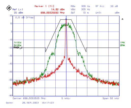
Plot # 10: Emission Mask J, , RF Output, Low Power Setting Frequency: 901 MHz, Modulation: 2-Level 8kbps GMSK
