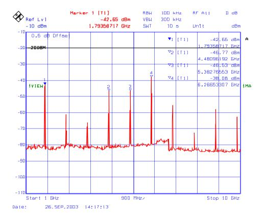
Plot # 19 : Spurious Emission Conducted at Antenna terminal, Low power setting Frequency: 898.5 MHz, Modulation: 2-Level 8kbps GMSK
