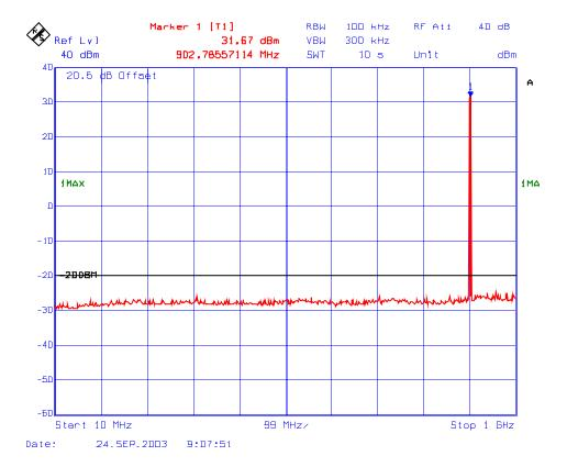
Plot # 16: Spurious Emission Conducted at Antenna terminal, High power setting Frequency: 901 MHz, Modulation: 2-Level 8kbps GMSK
