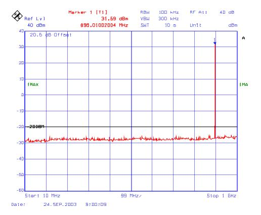
Plot # 12 : Spurious Emission Conducted at Antenna terminal, High power setting Frequency: 896 MHz, Modulation: 2-Level 8kbps GMSK
