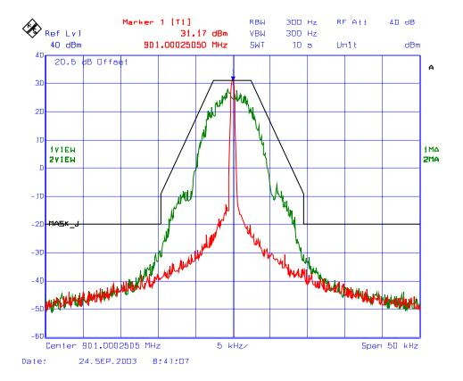
Plot # 8: Emission Mask J, , RF Output, Low Power Setting Frequency: 896 MHz, Modulation: 2-Level 8kbps GMSK
