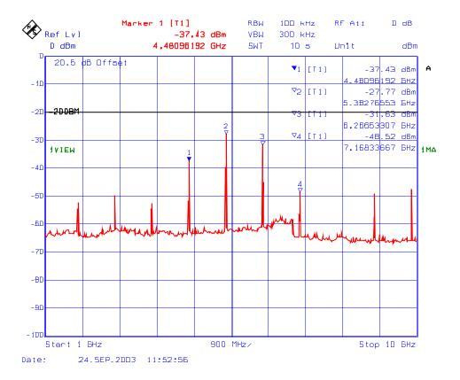
Plot # 13 : Spurious Emission Conducted at Antenna terminal, High power setting Frequency: 898.5 MHz, Modulation: 2-Level 8kbps GMSK
