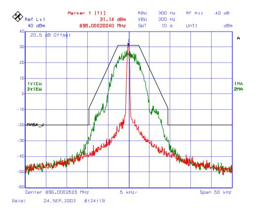
Plot # 6: Emission Mask J, , RF Output, High Power Setting Frequency: 898.5 MHz, Modulation: 2-Level 8kbps GMSK
