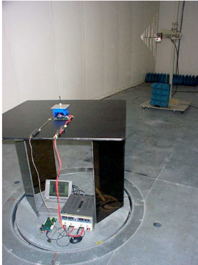
WaveNet BOOMER II (900 MHz) Wireless OEM Modem Module Testing for Spurious Emissions from Transmitter Frequency Range: 200 MHz – 1 GHz
