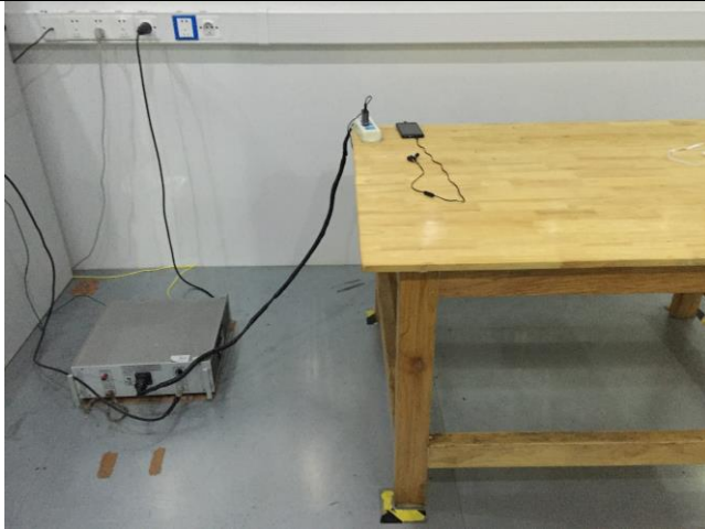
Conducted Emissions Test Setup Front View
