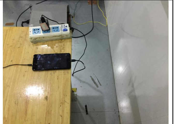
Conducted Emissions Test Setup Side View
