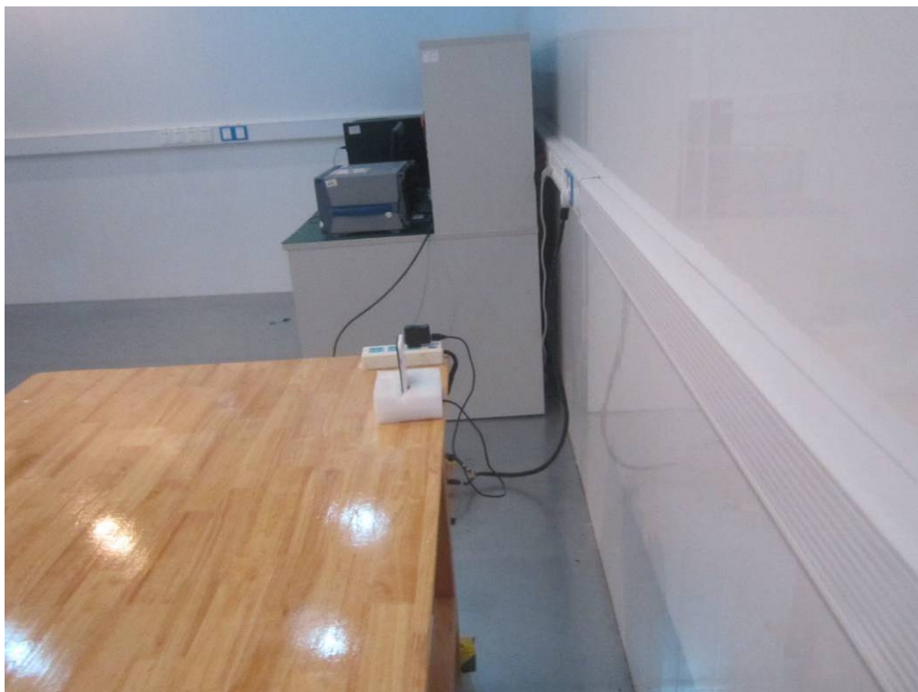
Conducted Emissions Test Setup Side View
