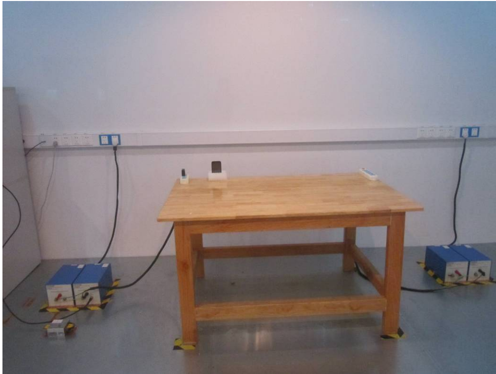
Conducted Emissions Test Setup Front View
