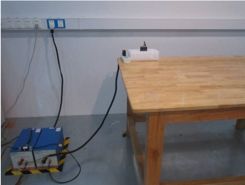
Conducted Emissions Test Setup Front View
