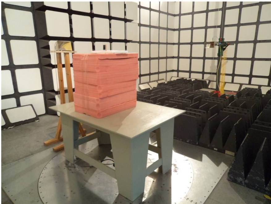
Radiated Emissions Test View – Above 1 GHz
