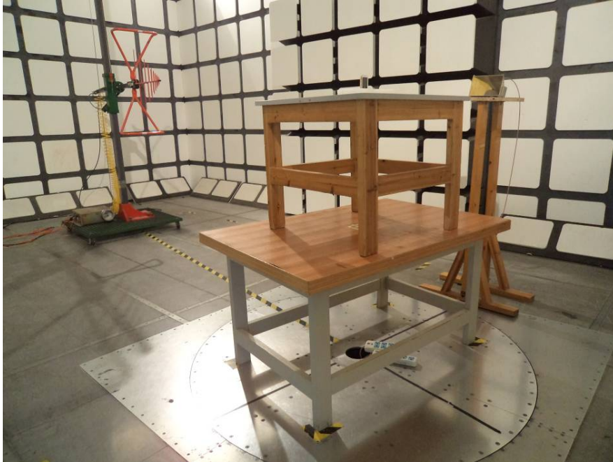
Radiated Emissions Test View – Below 1 GHz
