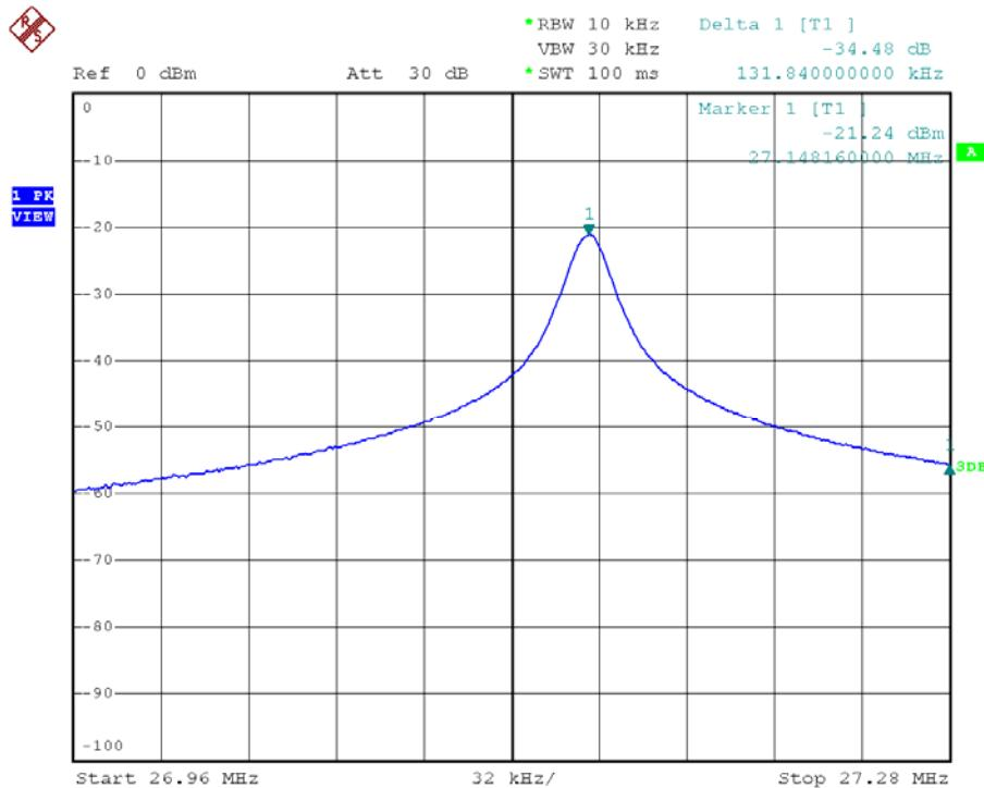
Bandwidth / Bandedge Plot – Pursuant to FCC Part 15 Section 15. 227 Requirement (Pass)
