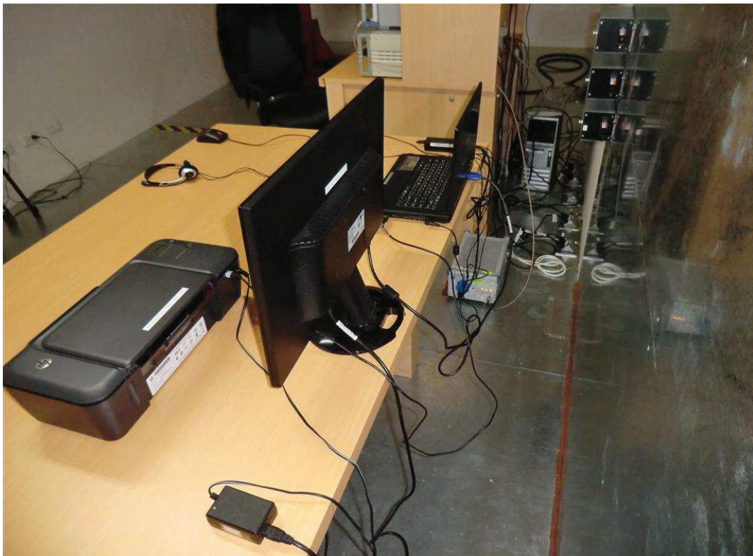
Photograph 6: Set-up for Mains Conducted Emissions (Back View)
