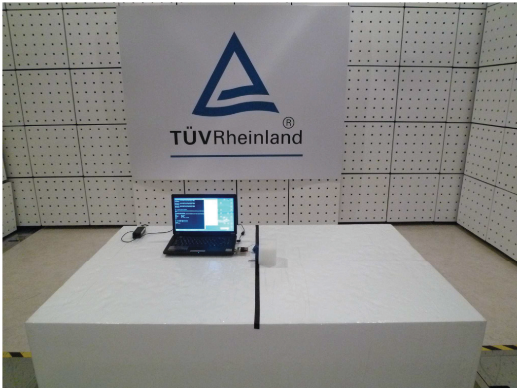
Photograph 2: Set-up for Spurious Emissions (Back View 1)
