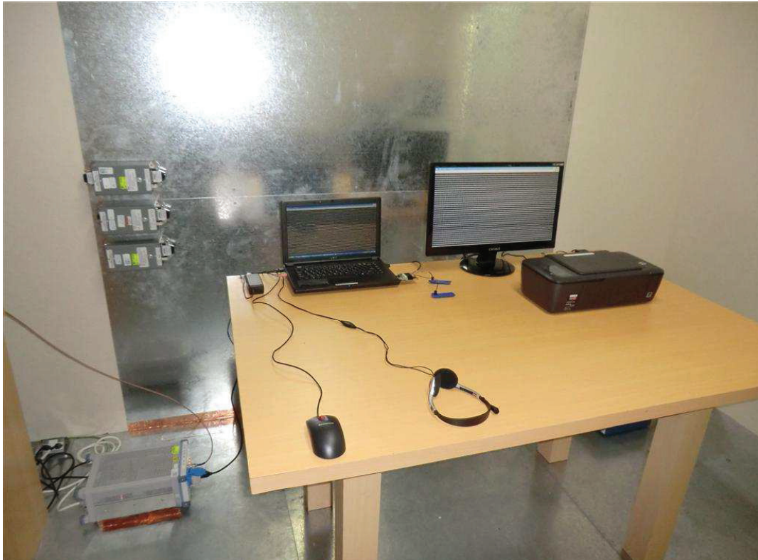
Photograph 6: Set-up for Mains Conducted Emissions (Back View)
