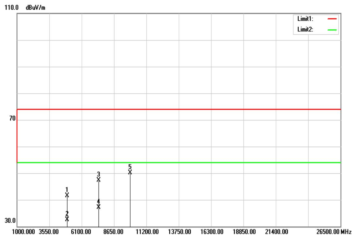
**Operation Mode:** GFSK / TX / CH High**Test Date:** November 15, 2016**Temperature:** 27°C**Tested by:** Dennis Li**Humidity:** 53 % RH**Polarity:** Ver. / Hor.
