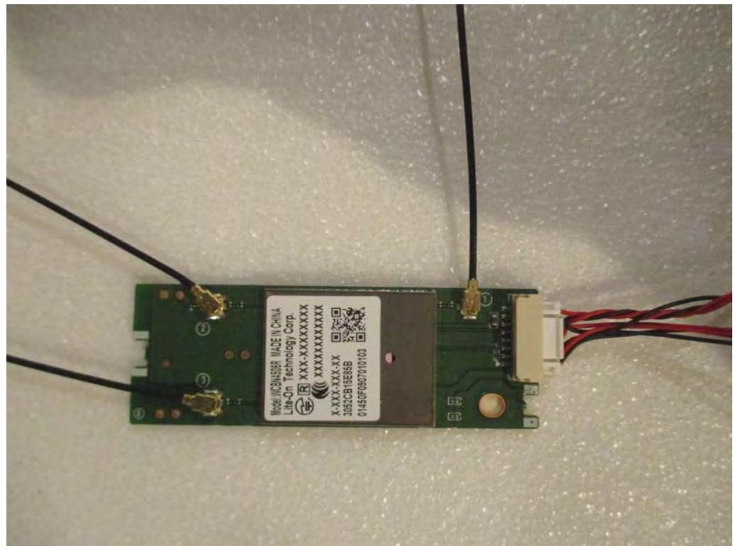
Place EUT 1 in Z axis + Set 2 antenna for 5G Band 3
