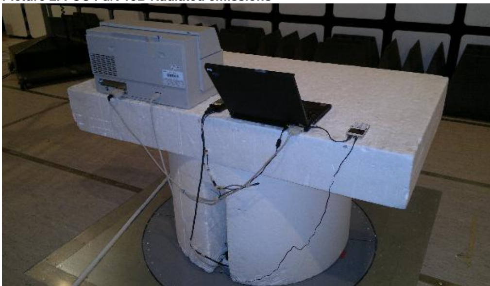
Picture 2. FCC Part 15B Radiated emissions
