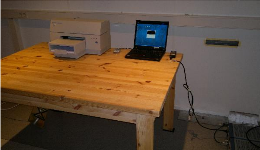
Picture 5. FCC Part 15B AC powerline conducted emissions from Mobile Charger
