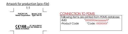
Blank label material: To be printed in NMP production using (600dpi) Thermal Transfer Printer Place tolerance of printing +/-0.3
