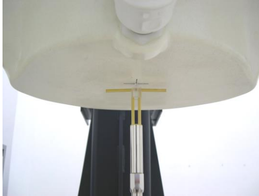
Fig 7.2 Photo of Dipole Setup
