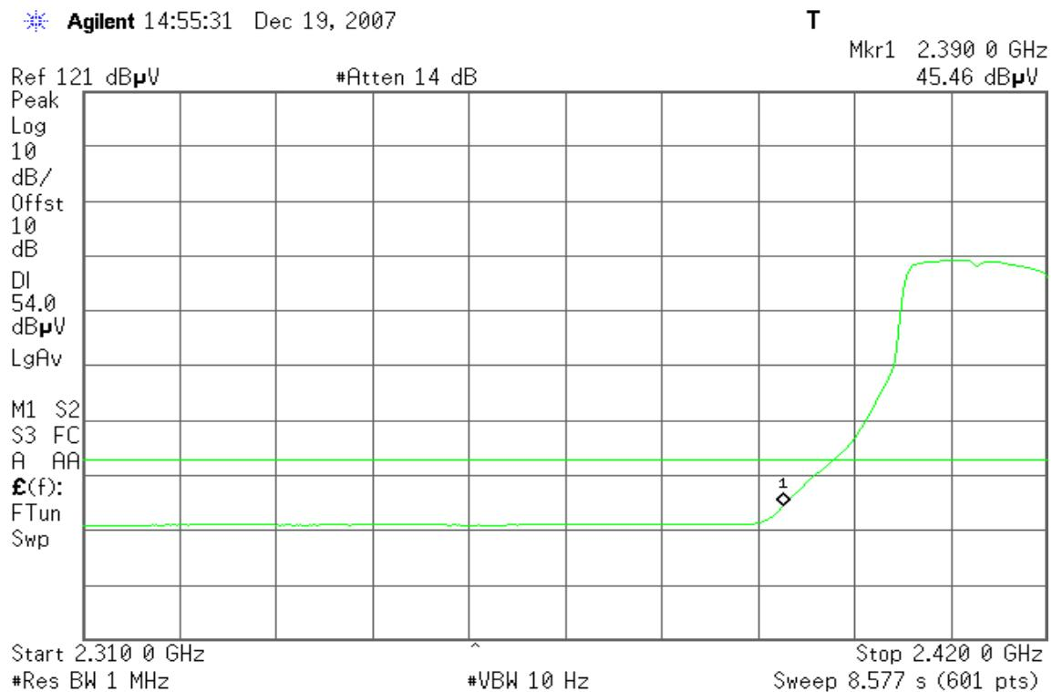
**Band Edges (IEEE 802.11g / CH High)****Detector mode: Peak****Polarity: Vertical**
