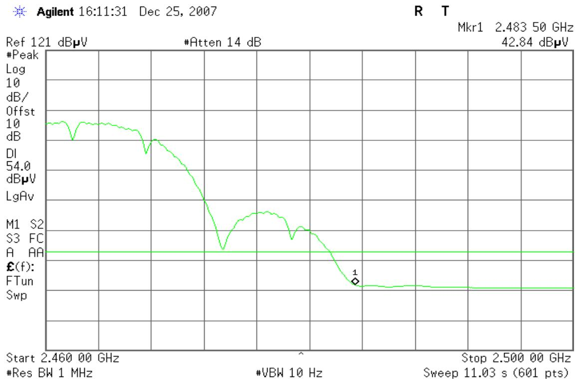
**Band Edges (IEEE 802.11g / CH Low)****Detector mode: Peak****Polarity: Vertical**
