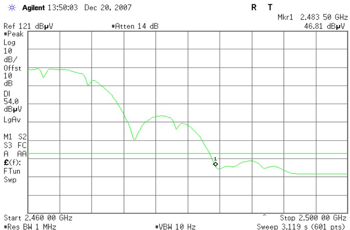
**Band Edges (IEEE 802.11g / CH Low)****Detector mode: Peak****Polarity: Vertical**
