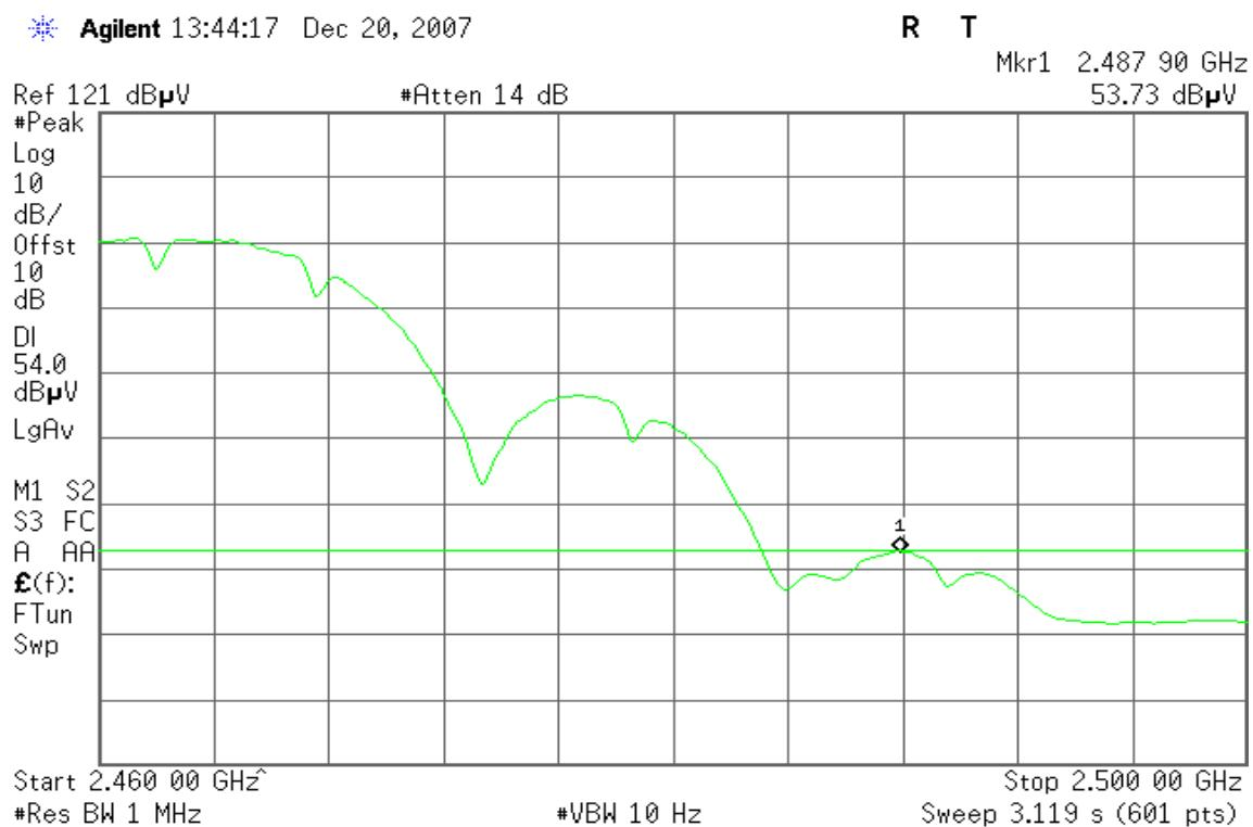
**Detector mode: Peak****Polarity: Horizontal**
