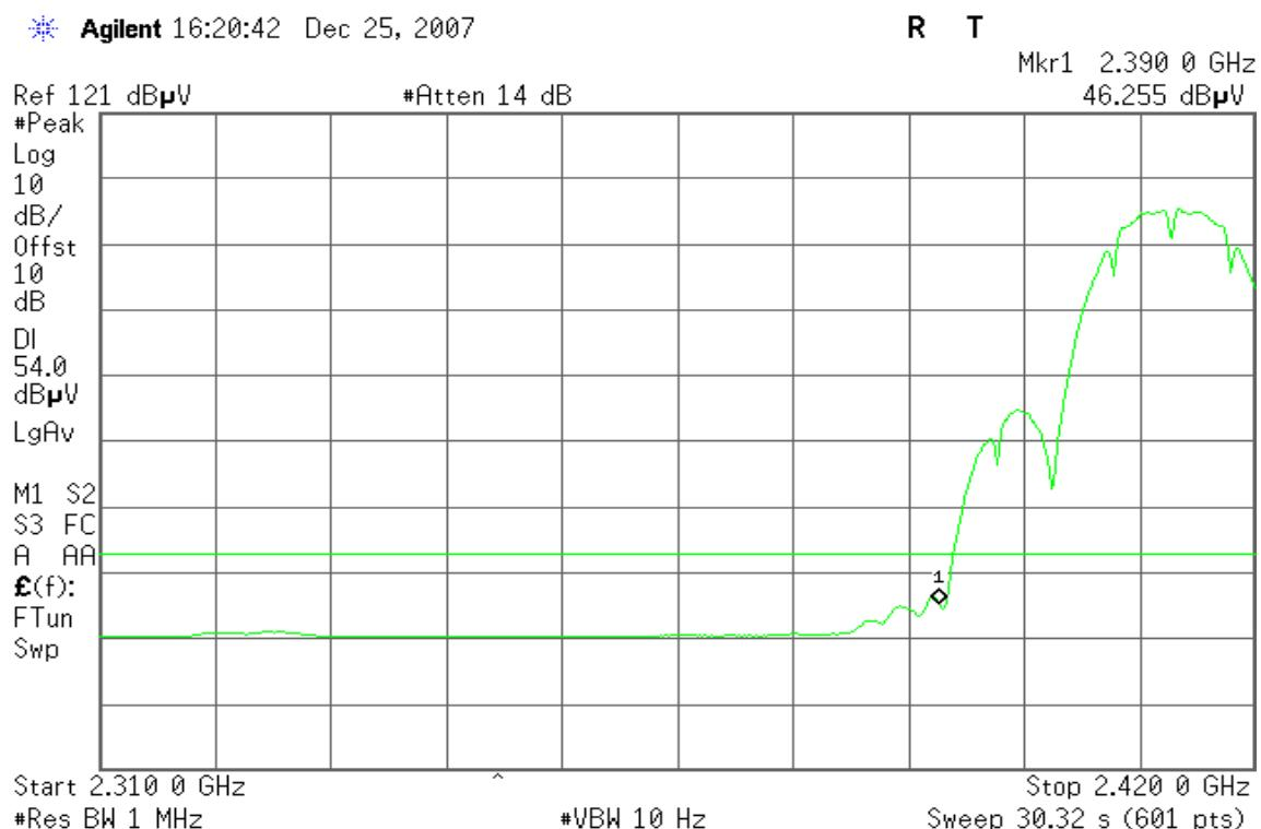
**Detector mode: Peak****Polarity: Horizontal**
