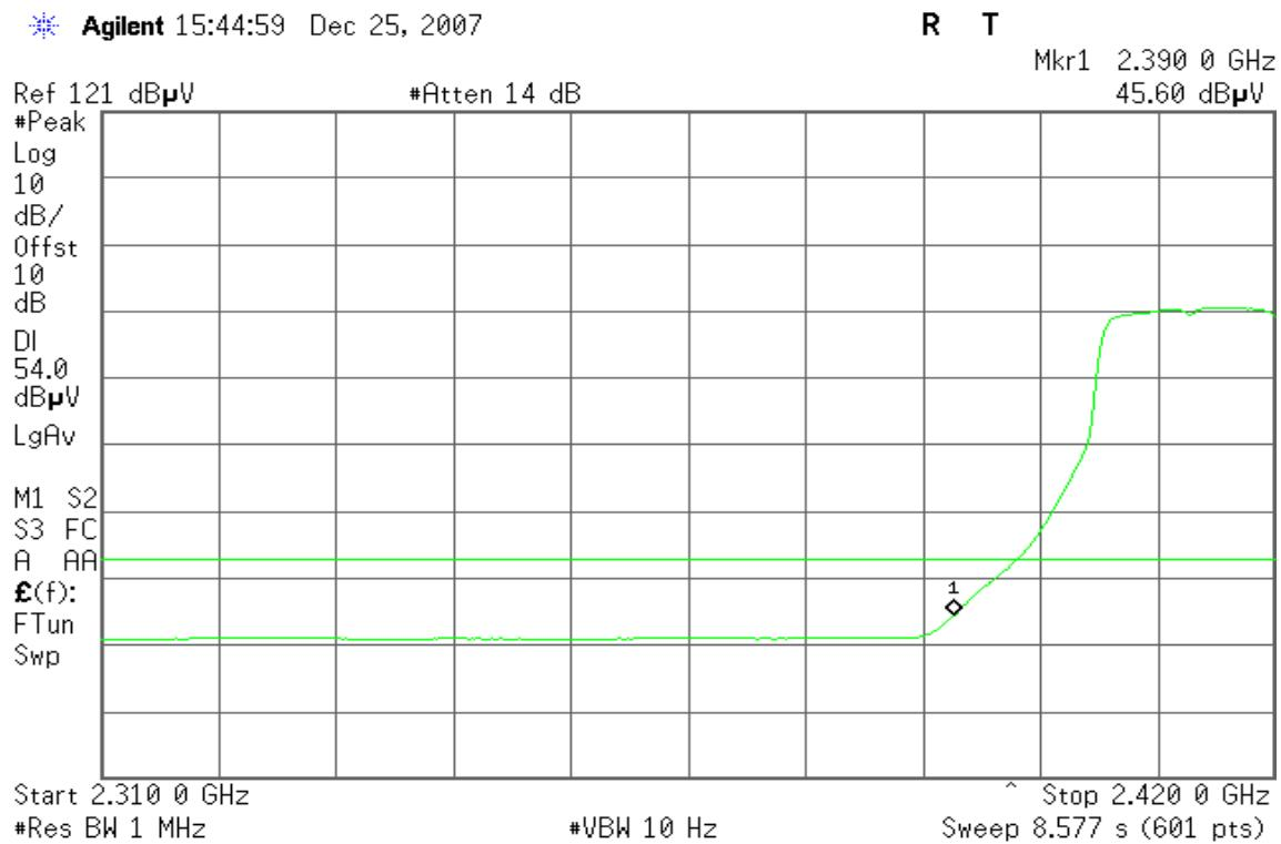
**Band Edges (IEEE 802.11g / CH High)****Detector mode: Peak****Polarity: Vertical**
