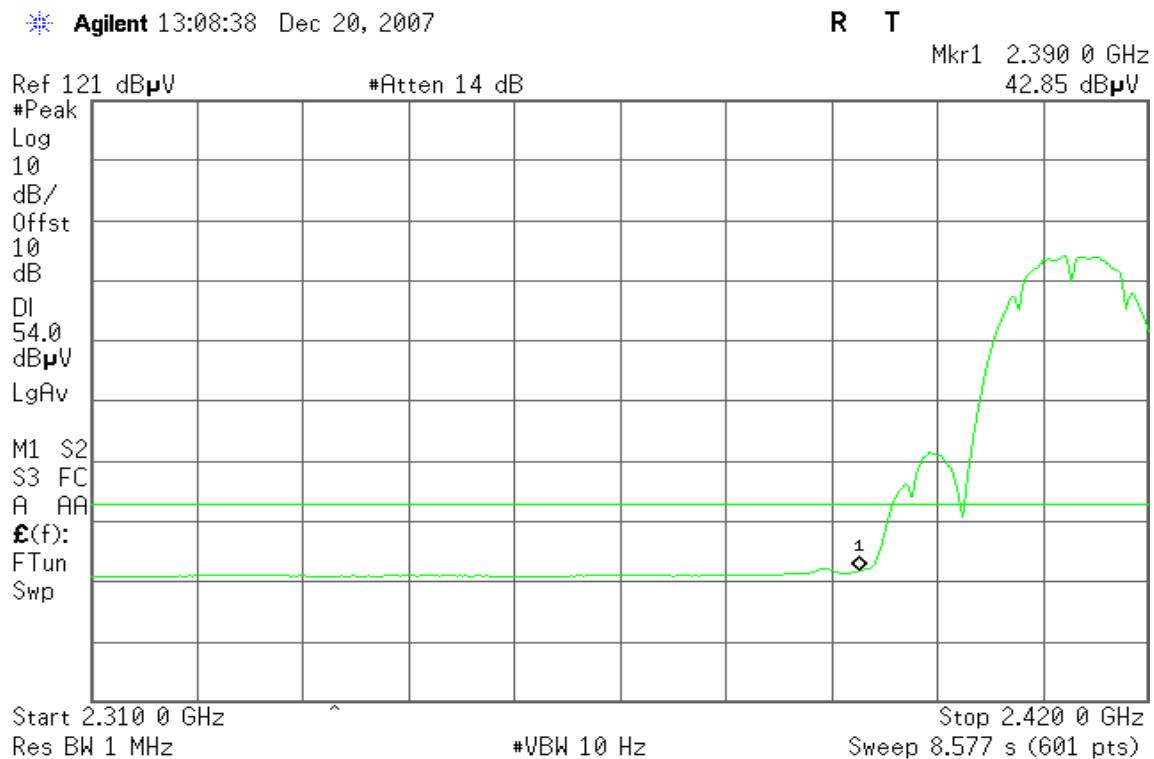
**Band Edges (IEEE 802.11b / CH High)****Detector mode: Peak****Polarity: Vertical**
