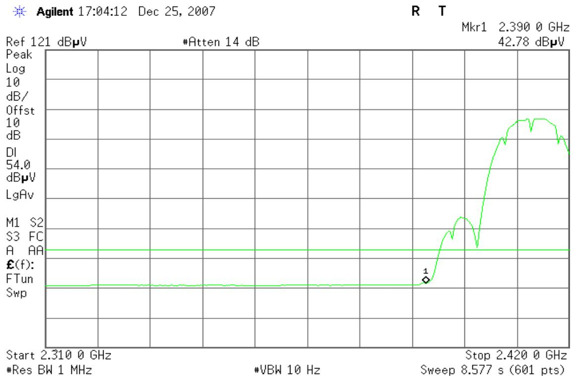
**Band Edges (IEEE 802.11b / CH High)****Detector mode: Peak****Polarity: Vertical**
