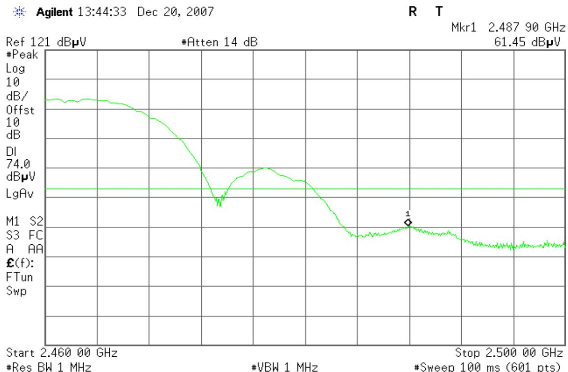
**Detector mode: Average****Polarity: Vertical**
