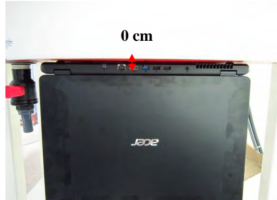
Fig.3 EUT Laptop mode to flat phantom
