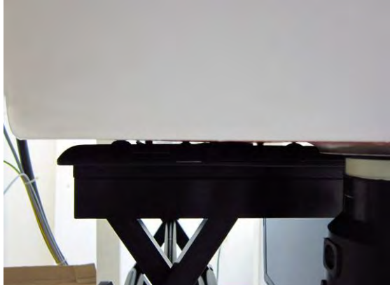
Fig.3 EUT Laptop mode to flat phantom
