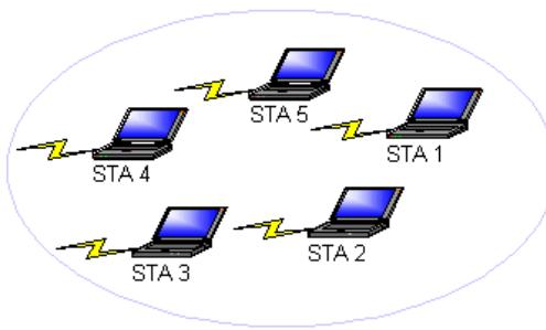
To connect to an ad hoc network, configure the profile for ad hoc mode. *Ad Hoc operation may be limited by Hardware to meet regulatory requirements.*
