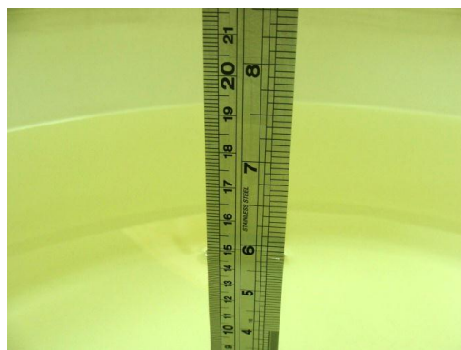
Fig 6.2 Photo of Liquid Height for Body SAR
