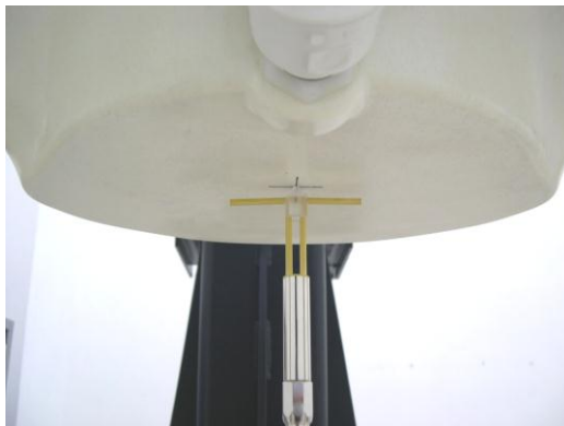
Fig 7.2 Photo of Dipole Setup
