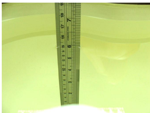
Fig 6.1 Photo of Liquid Height for Head SAR
