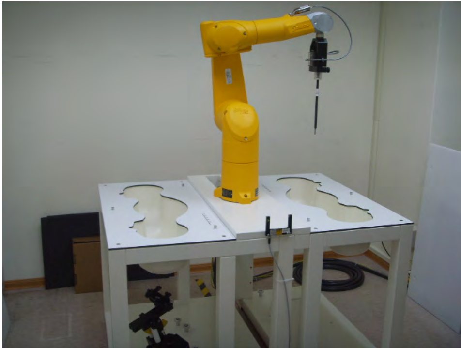
Fig.1 Photograph of the SAR Measurement System
