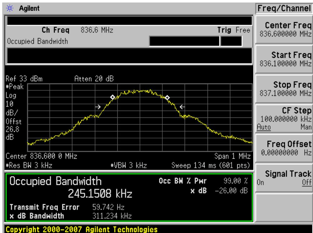
■ GSM850 MODE (251 CH.) Occupied Bandwidth
