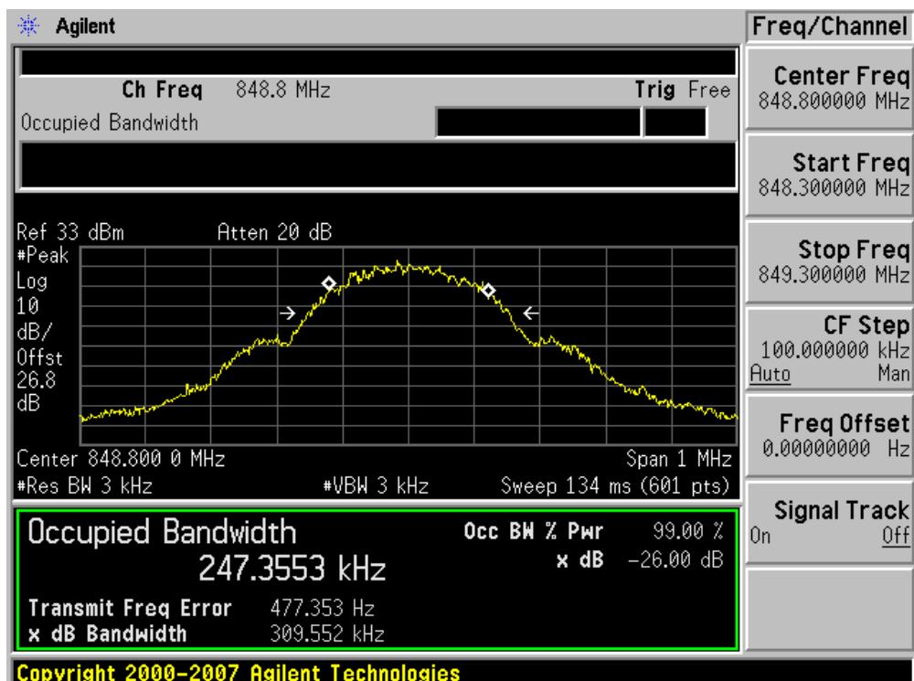
■ GSM1900 MODE (512 CH.) Occupied Bandwidth
