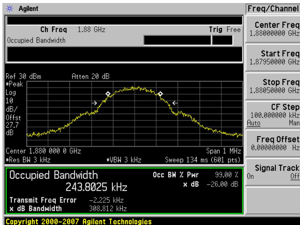
■ GSM1900 MODE (810 CH.) Occupied Bandwidth
