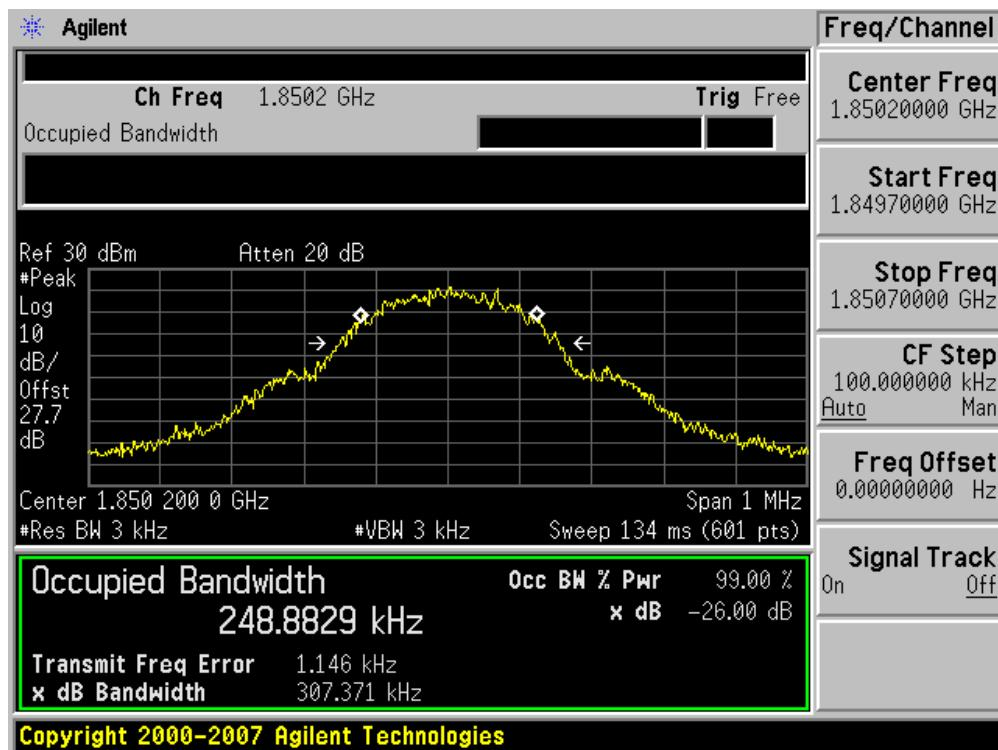
■ GSM1900 MODE (661 CH.) Occupied Bandwidth
