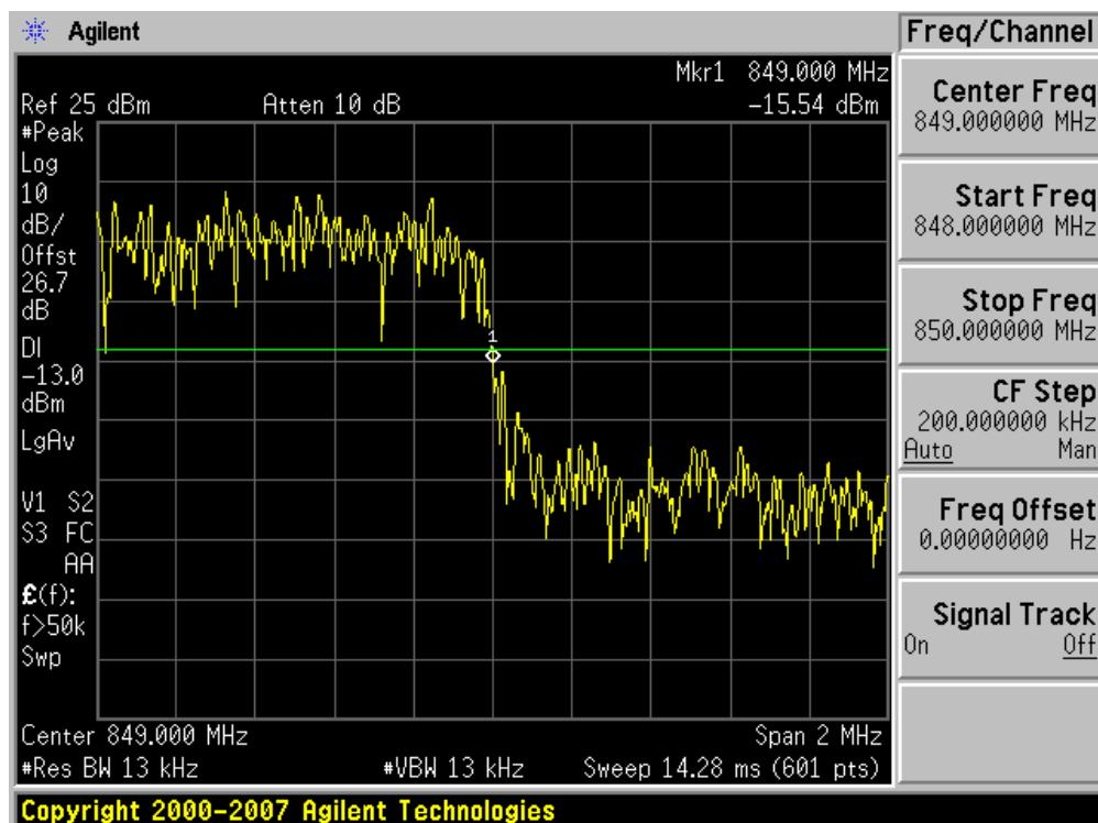
■ CDMA MODE (1013 CH.) 4 MHz Span - Block Edge
