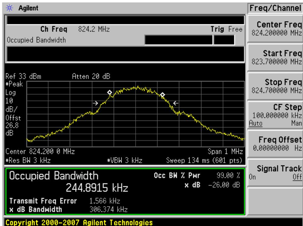
■ GSM850 MODE (190 CH.) Occupied Bandwidth
