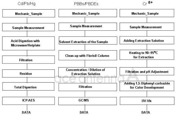
The samples were dissolved totally by pre-conditioning method according to above flow chart for Cd,Pb,Hg.
